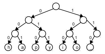
In the above tree, the encoding for 'y' can be determined by tracing the path from the root to the 'y' node. Going left then right again represents a 011 encoding.
